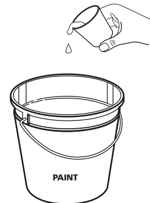
Latex Paint: Use Thin Layer of Water to Cover Paint
