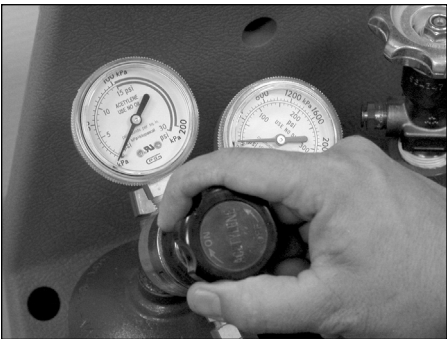
Figure 5 - Adjusting fuel cylinder valve
