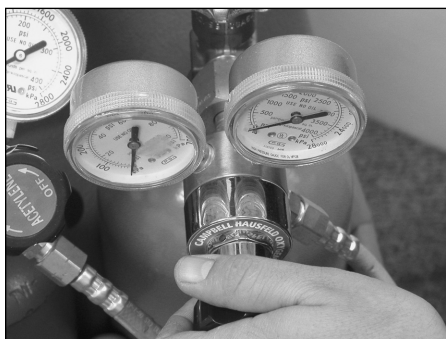
Figure 11 - Adjusting oxygen cylinder regulator
