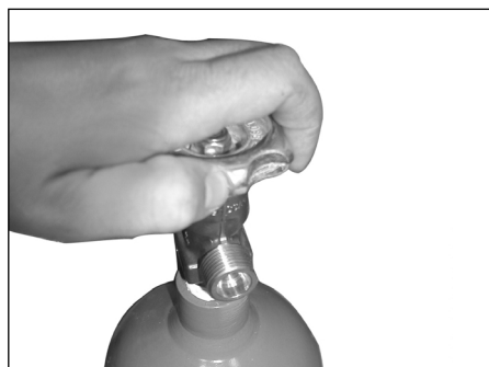
Figure 1 - Cracking the Cylinder Valve
