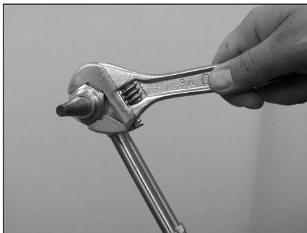
Figure 9 - Tightening cutting tip
