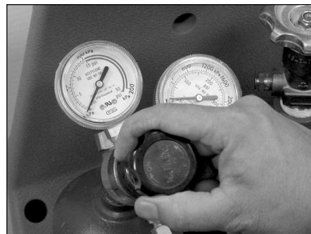
Figure 13 - Adjusting fuel cylinder regulator
