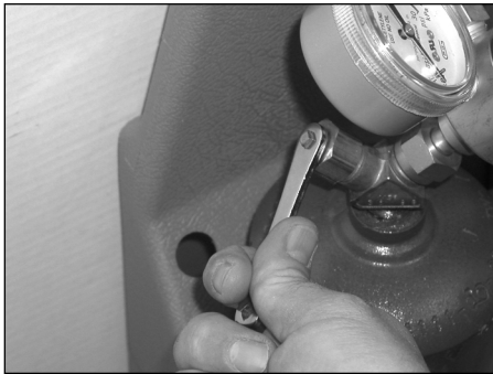
Figure 4 - Turning on gas
