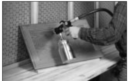
Spraying cabinet doors
