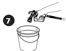
7 While Pulling Trigger, Direct Fluid Stream Along Inside of Bucket
