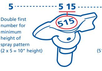
numbers indicate orifice size in thousandths of an inch (515 = .015" orifice)
