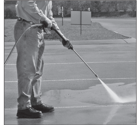
Figure 14 - Optimum angle to cleaning surface
