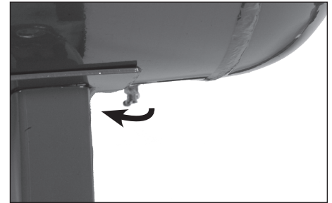
Figure 9 - Manual Tank Drain
