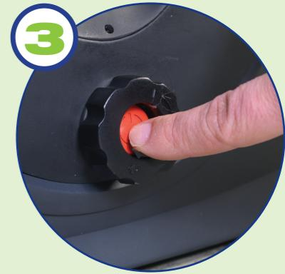
**Connect** universal adapter to valve stem. With universal adapter in place, **press** locking lever down.
