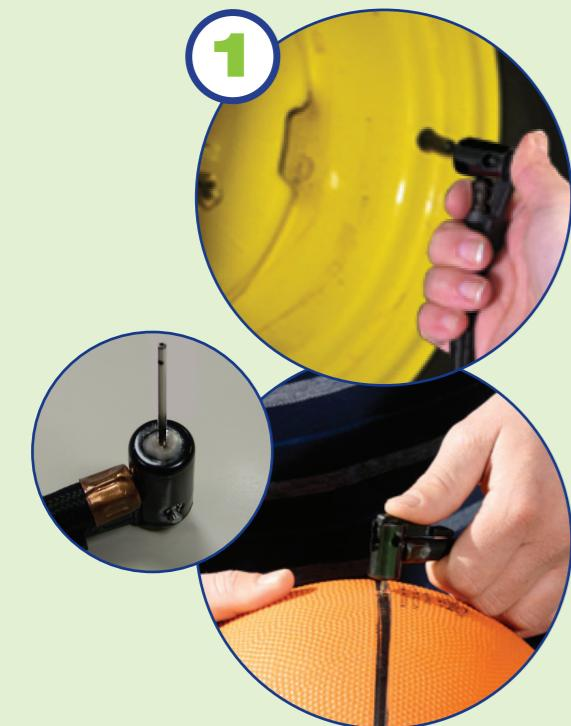
**Connect** universal adapter to valve stem **or Insert** inflation needle securely into the universal adapter. With universal adapter in place, **Press** locking lever down.
