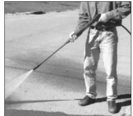
Figure 5 - Optimum Angle to Cleaning Surface
