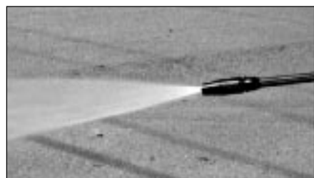
Figure 4 - Configuration éventail large
