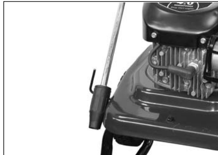
Figure 3 - Wire hanger on base plate
