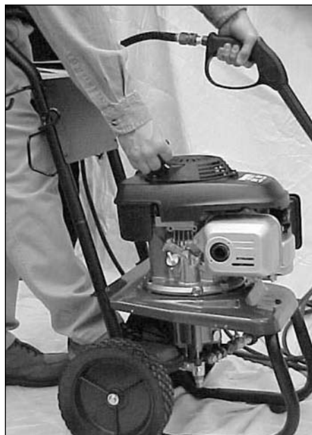
Figure 13 - Start the engine
