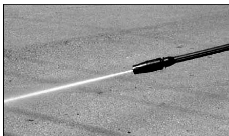
Figure 15 - Narrow high impact stream
