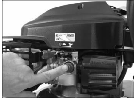
Figure 12 – Push the primer bulb 3 or 4 times
