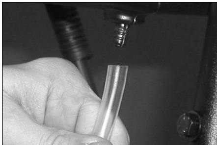
Figure 5 – Attach suction tube to barb fitting
