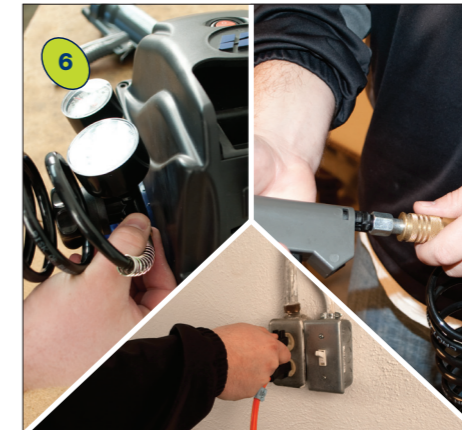
Attach air hose to air compressor and drain cleaner. Plug unit in.
