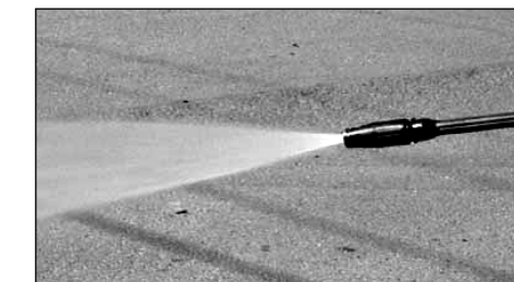
Figure 17 - Wide fan pattern
