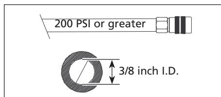
4. Use a pressure regulator on the compressor, with an operating pressure of 0 PSI - 125 PSI. A pressure regulator is required to control the operating pressure of the tool between 60 PSI and 90 PSI.
