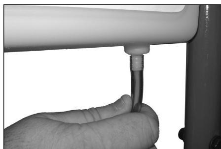
Figure 3 - Attach suction tube to barb fitting
