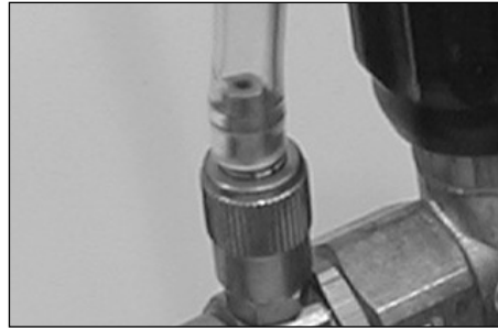
Figure 2 - Attach suction tube to barb fitting
