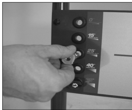
Figure 3 - Insert spray tips into the holder
