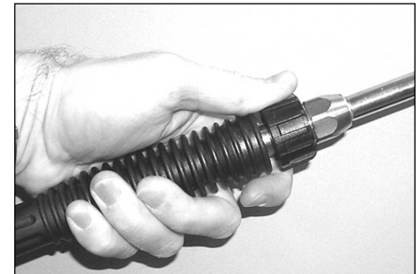
Figure 6 - Attach lance to gun
