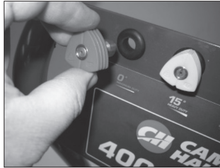
Figure 3 - Insert spray tips into the holder
